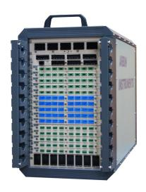
Available auxiliary chassis allows connectivity for auxiliary temperature and voltage measurements as well as analog input/output modules for interaction and control of third party devices.
