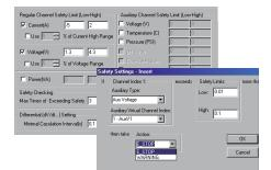
• The user is able to implement safety limits in the software for current, voltage, total power, as well as temperature or other auxiliary readings. These values can be programmed to send the system into a rest state for a period of time, or simply stop the test and disconnect the charge/discharge circuitry. There are separate limits available for each test schedule as a whole, and individual steps within the test schedule.
