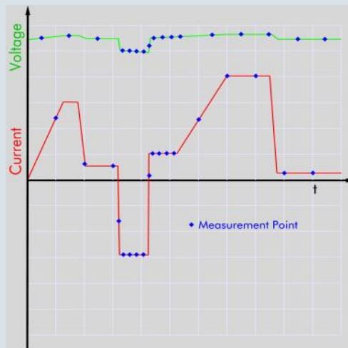
Synchronized data logging with variable scanning rate for waveform. Simultaneous measurement of voltage and current.
