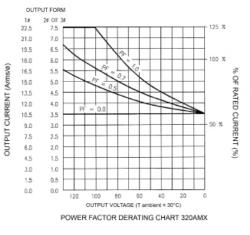
OUTPUT VOLTAGE-AC VOLTS RMS
