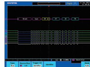
LIN Bus Trigger and Decoding Function
