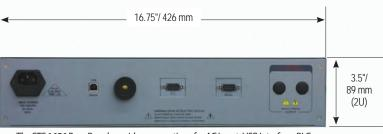
The STS 1656 Rear Panel provides connections for AC Input, USB interface, PLC I/O and RS232 interface option.
