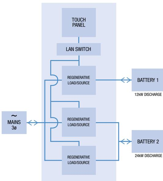
Figure 1 - Independent testing of 2 different battery types
