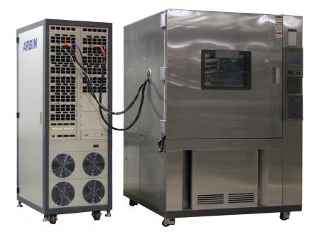
The Arbin BT-ML series is a high precision testing solution designed for testing modules and small packs of batteries and/or supercapacitors. Today's applications like electric vehicles and military technologies demand high-reliability and safe testing environments, so the dependability, accuracy, and safety of these systems are core standards. A full range of optional customizations allow users to create a complete testing package that ideally suits their needs.
