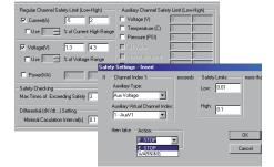
The user is able to implement safety limits in the software for current, voltage, total power, as well as temperature or other auxiliary readings. These values can be programmed to send the system into a rest state for a period of time, or simply stop the test and disconnect the charge/discharge circuitry. There are separate limits available for each test schedule as a whole, and individual steps within the test schedule.
