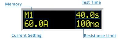
Follow the setup procedures to set the desired parameters. The display will show the Ground Bond test settings depending:
