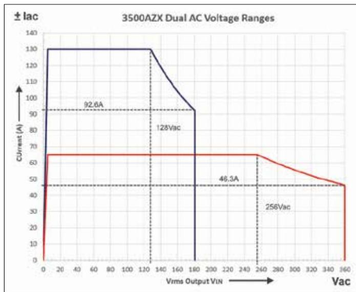
High and Low AC Voltage Range Constant Power Profiles - 50kW Model.
